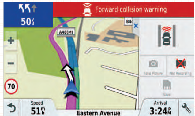
Forward Collision Warning – Alerts if you drive too close to the car ahead.
