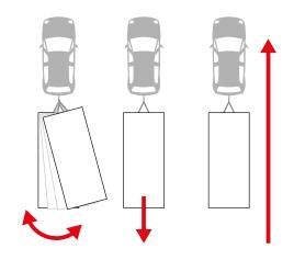
The driving behaviour of the trailer is permanently monitored by the ATC. Sensors detect dangerous lateral movements directly on the trailer axle, even before an ESP system for trailers installed in the car is able to sense the pendulum movement. The trailer will immediately – without any action on the part of the driver – brake gently and return to a stable driving condition.
